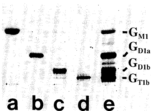
Fig. 3. Thin-layer chromatogram of individual gangliosides isolated from mouse brain by preparative TLC using NBD dihexadecylamine dissolved as reversible stain in the running solvent. Gangliosides were chromatographed in chloroform-methanol-20 mM aq. \text{CaCl}_2 (120:85:20, v/v/v) and visualized by spraying the plate with resorcinol-HCl reagent. Aliquots of TLC purified G_{M1} (a), G_{D1a} (b), G_{D1b} (c), G_{T1b} (d) and 15 \mu\text{g} of whole gangliosides from mouse brain (e) were applied [73].
